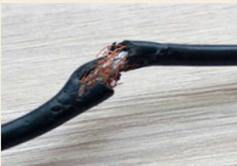
Figure 8.0: This figure shows the damage caused by rodents
